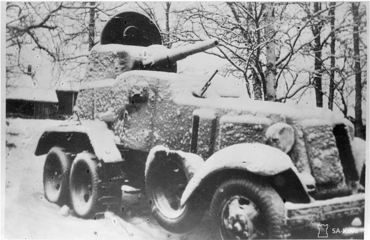
A BA-10 armored car fitted with the optional half-tracks over the rear wheels (SA-Kuva).
