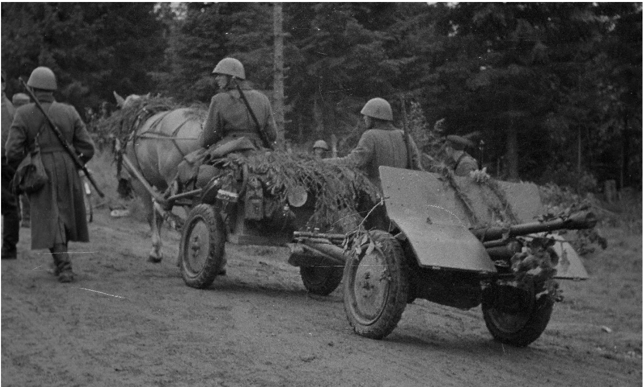
The 37mm Bofors AT gun pictured during the Continuation War. Note that a single horse is sufficient for pulling the gun and limber. The crew is walking, and the lower plates of the gun shield have been folded up during transport (SA-Kuva)
