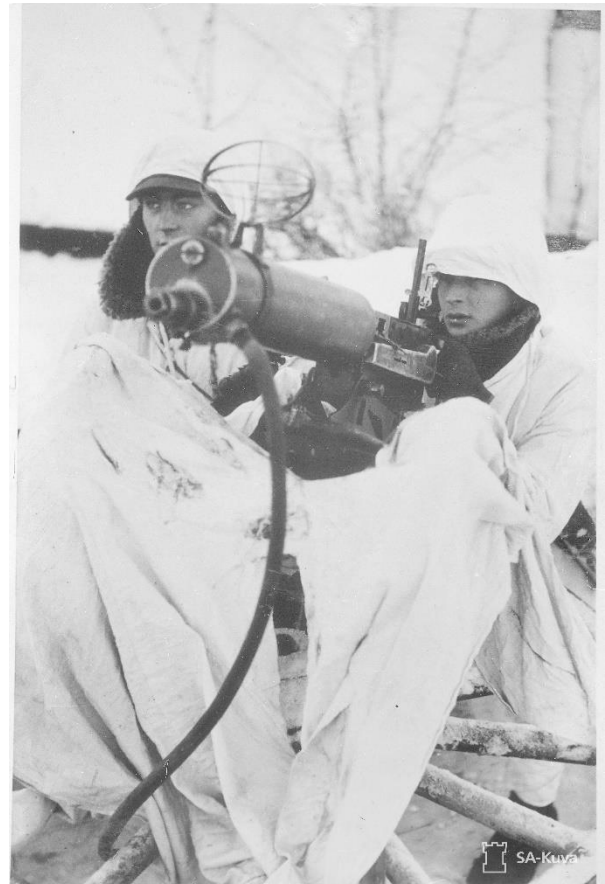
A model 09-21 Maxim MMG mounted on a cartwheel for anti-aircraft use (SA-Kuva)
